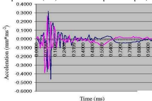
Fig. 6. Time variation for the acceleration of 2 points, belonging to the median line of the impact surface.
