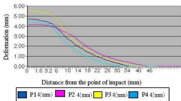
Fig. 2. Mean values of measured deformation on the posterior surface
