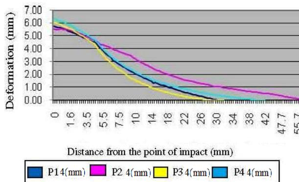
Fig. 1. Mean values of measured deformation on the impact surface
