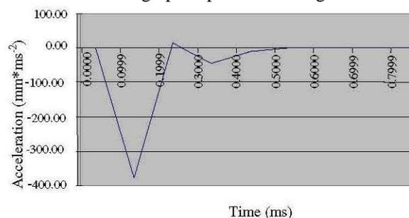
Fig. 4. Acceleration graph at the point of impact
