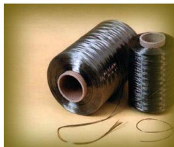
Fig. 1. Bobbins of basalt roving [12]
