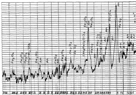
Fig. 2. Diffractogram of a sintered basalt part [11]
