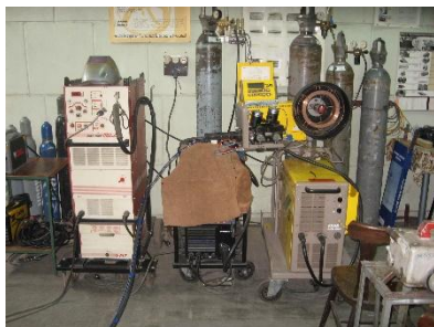
Fig. 1. Mechanised wire feed based WIG welding plant
