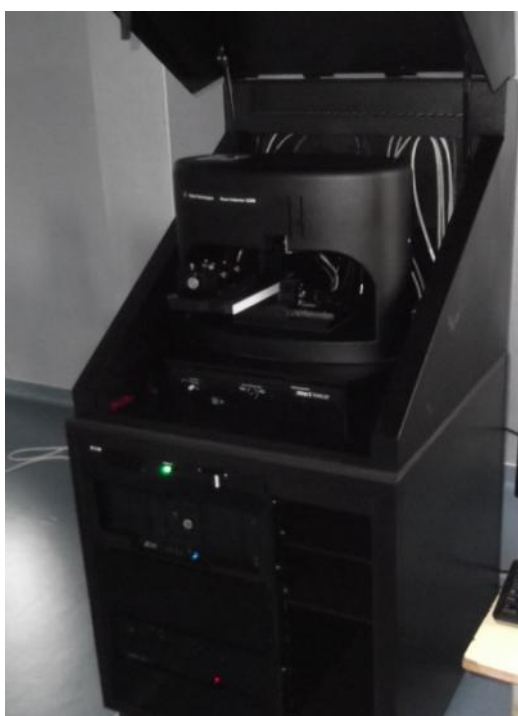
Fig. 2. The G200 nanoindenter in the SMARTMAT laboratory.
