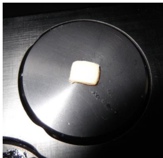
Fig. 3. The ceramic sample on the motorized stage of the G200 nanoindenter.
