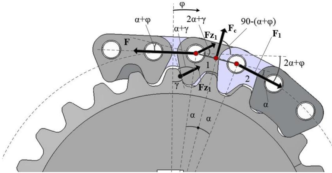
Fig. 2. Force distribution on silent chain transmission
