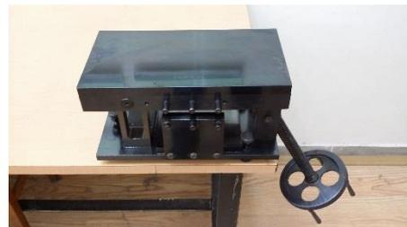
Fig. 1. Prismatic tribometer
