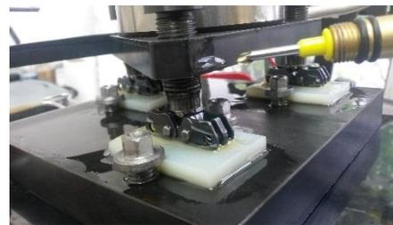
**Fig. 7.** Prismatic tribometer
