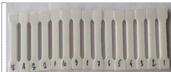
**Figure 5.** Samples printed for tensile testing.
