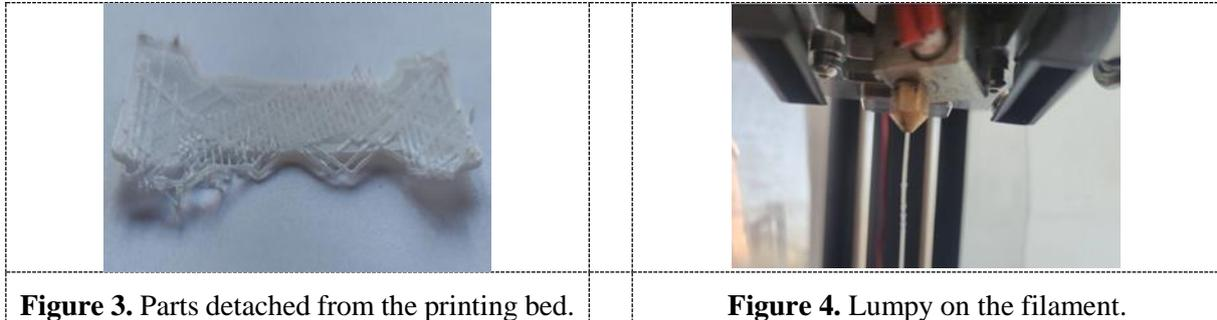
In the settings for the Delta printer, with the use of PLA filament, a printing temperature of 225°C was reached, a set speed of 85mm/s for the initial samples, the printing temperature for bed of 60 °C, and for the first layer was set the temperature of 210°C, because the speeds at this layer are up to 24.5mm/s.
