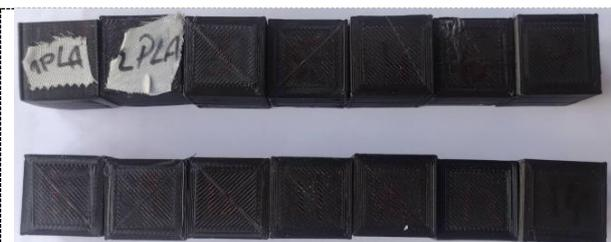
**Figure 6.** Samples for compressive testing.
