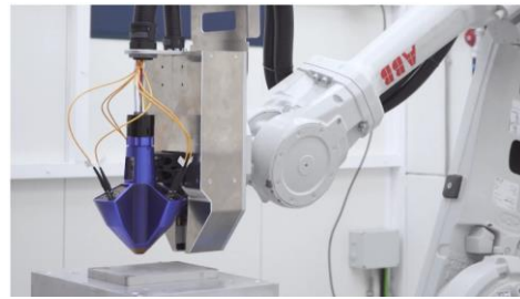
Figure 7. Mounting the Melted Engine head on an ABB robot [10]
