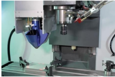
Figure 6. Meltio Engine print head fixed on a CNC [10]
