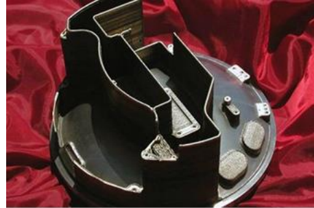
Figure 3. Part obtained by printing + milling in 3 weeks compared to 52 weeks with another method [8]
