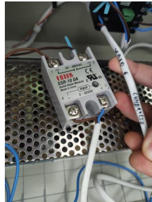
Figure 4 Wiring diagram - connecting the Figure 5 SSR mounted in the control panel printhead to the CNC
