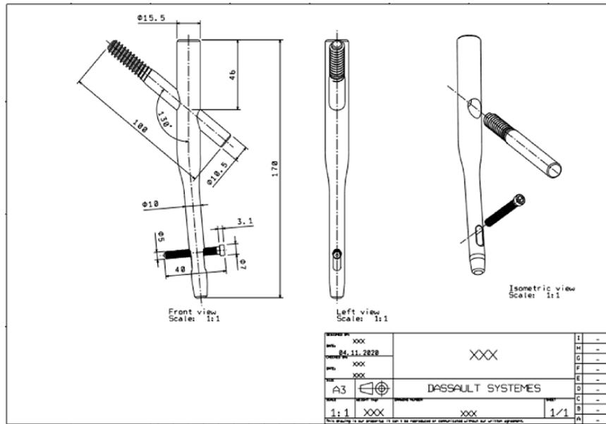
**Figure 1.** Execution drawing of the implant
