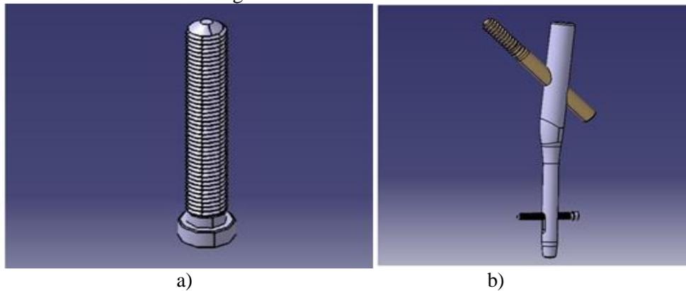
**Figure 3.** a) CAD model of the distal screw of the Gamma rod; b) The assembled CAD model of the Gamma rod
