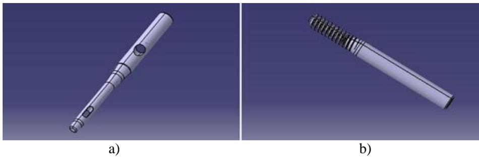
**Figure 2.** CAD model of: a) Gamma rod; b) the proximal screw of the Gamma rod
