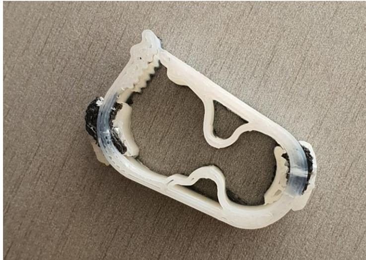
**Figure 4.** Flow regulator used for artificial respirators and also for intravenous infusion kits – this one was made on a 3D printer in our laboratories at University of Oradea
