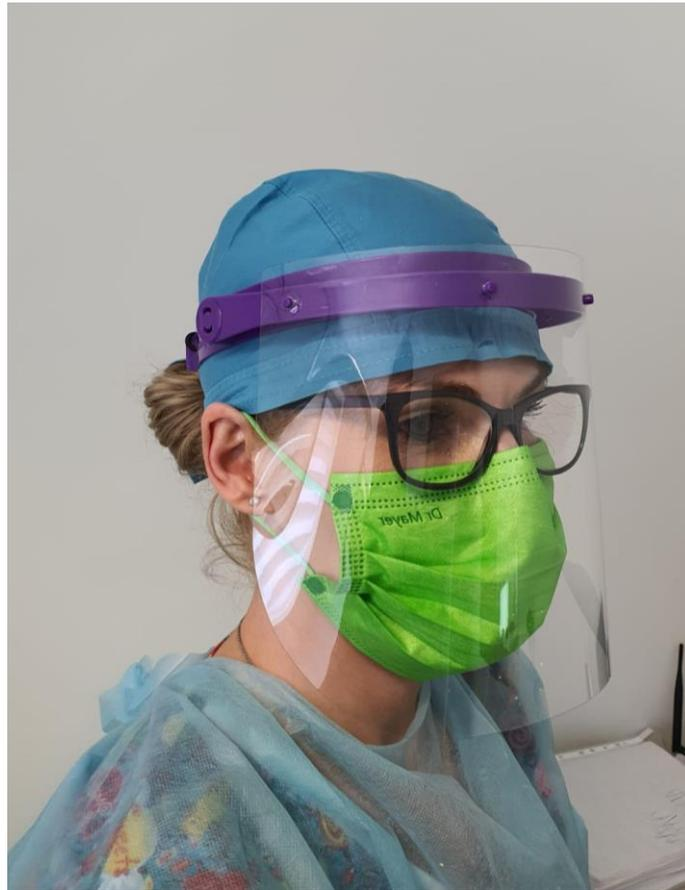
**Figure 3.** Face-shield used by medical practitioners made with the help of 3D printer – the plastic head support was made with the help of additive manufacturing than the transparent foil was mounted on the front clips.
