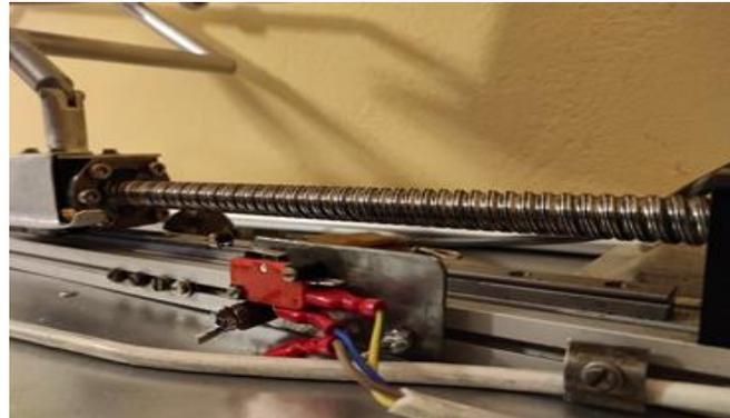
**Figure 14.** Mounting the limit switches.
