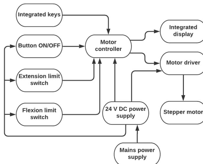
**Figure 1.** CPM device block diagram.
