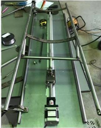
**Figure 10.** Mounting the motor and linear platform. **Figure 11.** Welding the support.
