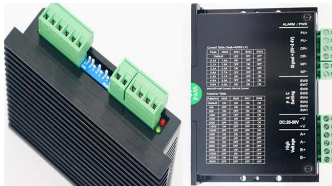
Figure 3. Motor Driver Nema 23 [6].
