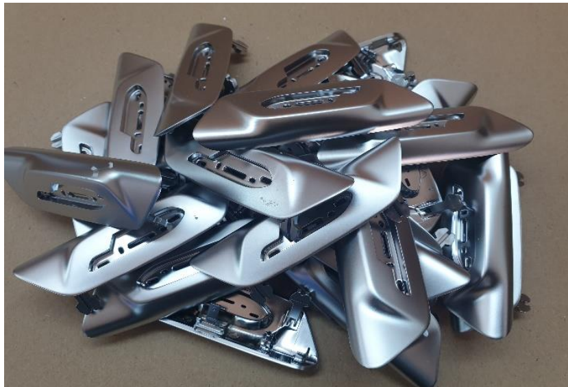
Figure 4. Sample with plated areas of 60-350 mm 2 , with layers of Cr 0,5-1 μm , Ni 40-70 μm and Cu 50-120 μm.
