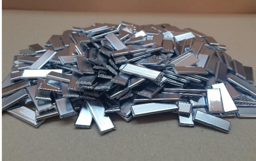
Figure 3. Sample with plated area of 50-60 mm 2 , with layers of Cr 0,5-1 μm , Ni 40-70 μm and Cu 50-120 μm.
