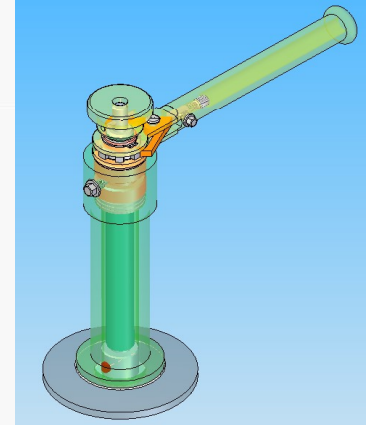
Fig.12. Jack-screw with rotating nut assembly
